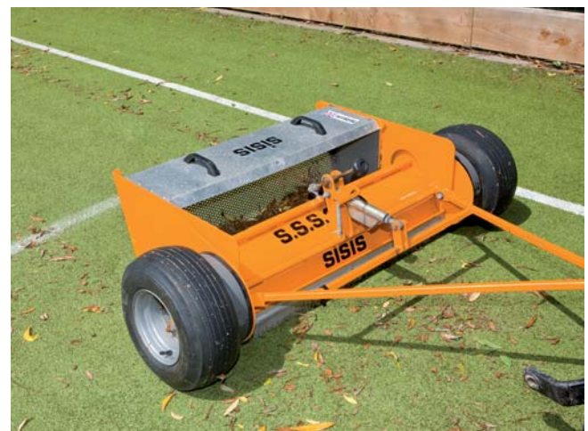
Figure 15: rotating brush to remove debris from the surface
