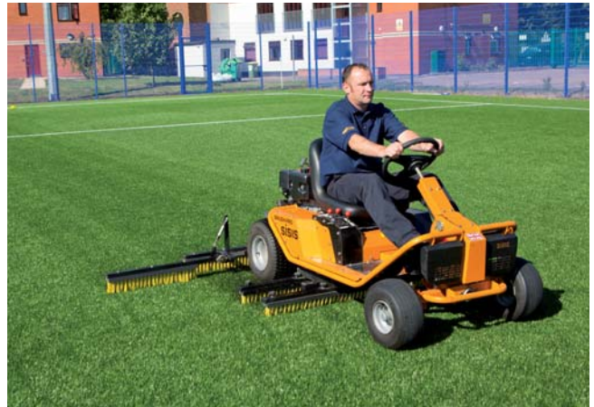
Figure 12: oscillating brush to bring the fibres upright
